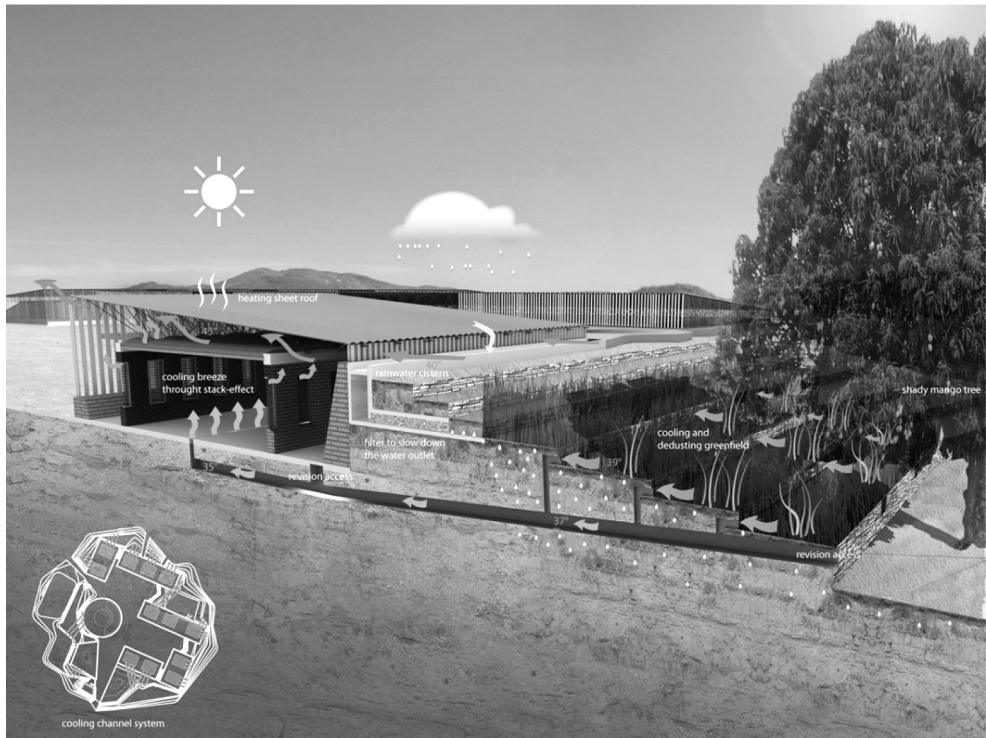
III. 8. Lower secondary school in Gando. Burkina Faso. Schematic natural ventilation school (source: [6])
