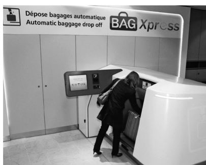
Ill. 3. ALSTEF baggage control system – the identification and marking of the baggage is performed in a self-service manner. The system requires adjustments, re construction and architectural design of “check-in” to meet new solutions (source: ALSTEF advertising materials, http://www.alstef.com )
